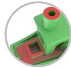
The top surfaces of the deck, box and chimney are planar, horizontal and parallel to the bottom plane.
