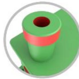
The chimney is designed to define concentric cylindrical shapes with inner and outer diameters. These clearly show deviations in roundness.
