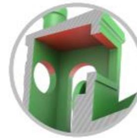
Overhang issues are the Achilles' heel of 3D printing. #3DBenchy offers several challenging areas such as in the difficult-to-reach inside of the bridge.
