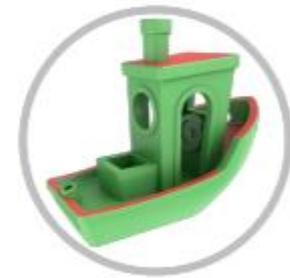
Low-slope-surfaces clearly show the layered structure of 3D printing. If printed horizontally, #3DBenchy's gunwale and roof of the bridge will reveal the layer-steps.
