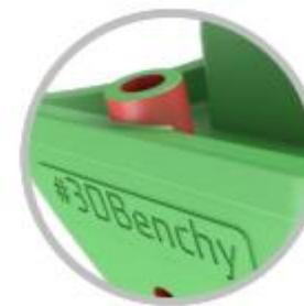
The fishing-rod-holder provides a very small slightly-slanted blind hole.
