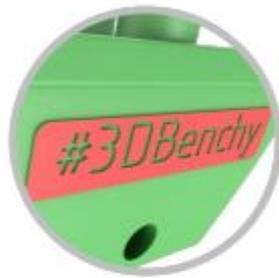
If you have a high-resolution 3D printer, this is where you can shine! The letters on the stern are less than 2 mm tall and the thickness of #3DBenchy's nameplate is just 0.1 mm.
