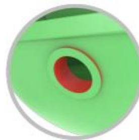
The hawsepipe represents a small short horizontal hole and has a very thin flange against the hull.
