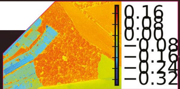
But it meant the red and infrared data would be saved to the same channel, making it impossible to distinguish the latter. “We had to improvise by using an alternative index (GLI), which compares the green channel to the red channel (G-R)/(G+R),” Oliver reveals.
