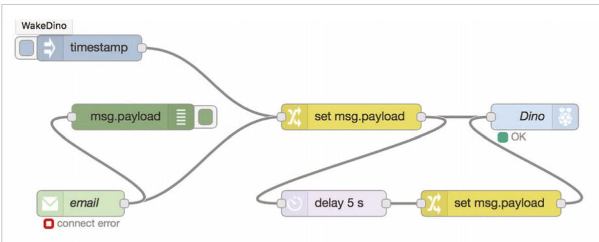
**Left** This Node-RED flow will trigger if any email is received. The delay node stops the dino after five seconds
