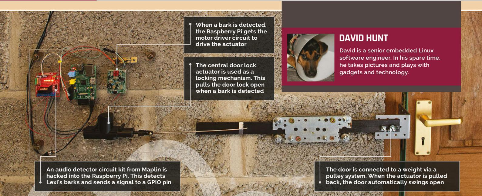
When a bark is detected, the Raspberry Pi gets the motor driver circuit to drive the actuator
