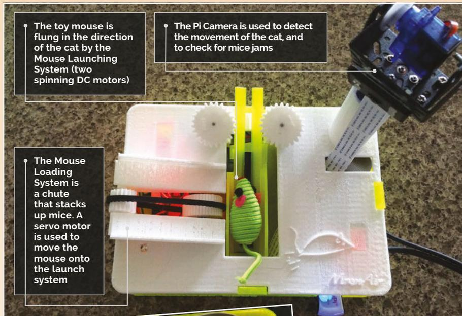
The toy mouse is flung in the direction of the cat by the Mouse Launching System (two spinning DC motors)
