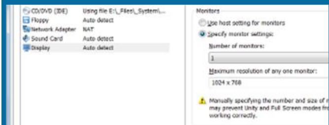
8. Finally, to allow Puppy to sit comfortably within a window, we can force the virtual screen to be a fixed size, ideally slightly smaller than the monitor you are using. So, for a 1280x1024 monitor, 1024x768 is fine.
