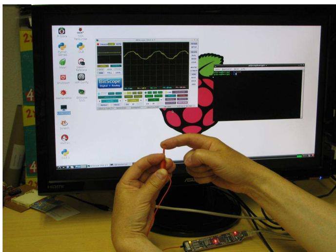
**Figure 4:** Touching the test lead with your fingertip
