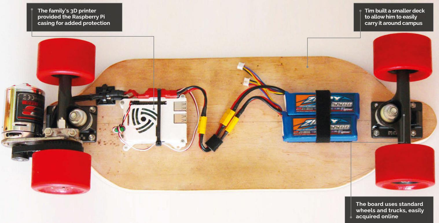
The family's 3D printer provided the Raspberry Pi casing for added protection
