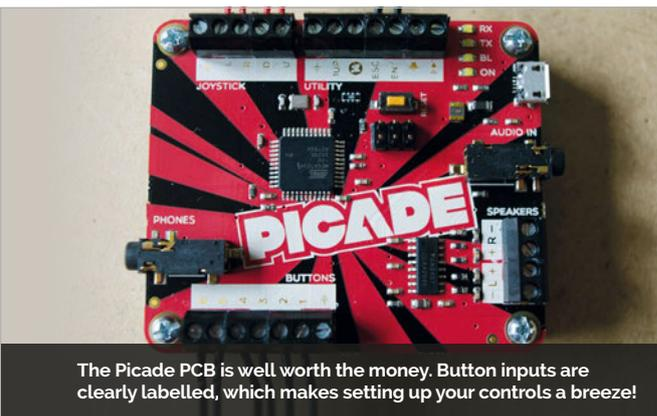
The Picade PCB is well worth the money. Button inputs are clearly labelled, which makes setting up your controls a breeze!
