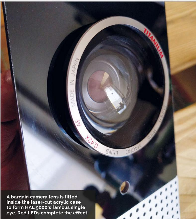
A bargain camera lens is fitted inside the laser-cut acrylic case to form HAL 9000's famous single eye. Red LEDs complete the effect
