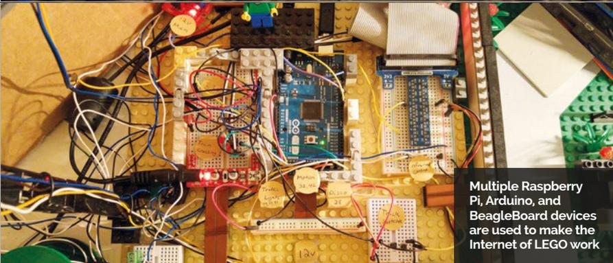
Multiple Raspberry Pi, Arduino, and BeagleBoard devices are used to make the Internet of LEGO work
