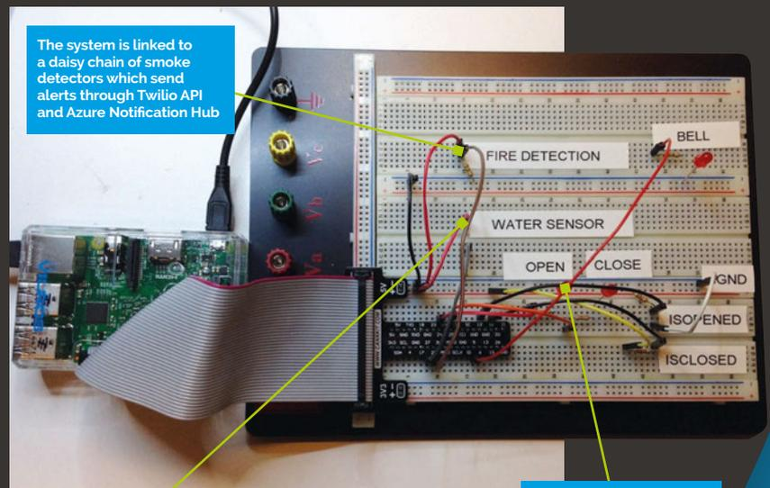
The system is linked to a daisy chain of smoke detectors which send alerts through Twilio API and Azure Notification Hub
