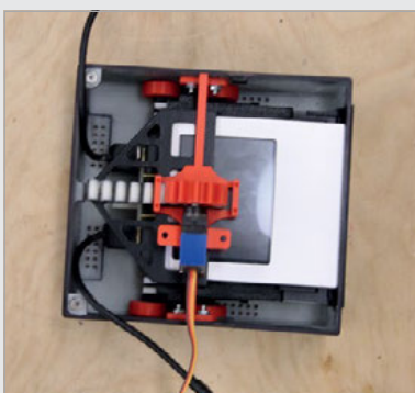
Right The cartridge looks like a Polaroid picture, and is ejected using a rack-and-pinion mechanism
