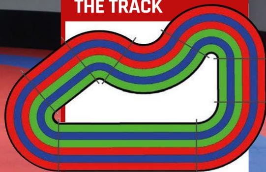
A purpose-built, brightly coloured track atop the PiBorg offices will be used for the racing series. The colours and slower speed of the robots allow for the camera on the YetiBorg to do some image processing while navigating the course.
