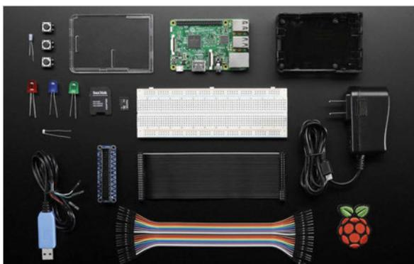
Electronic components are plugged into the holes on the breadboard, and components in adjacent holes are linked. In this way, you can build up a test circuit without having to actually solder components together.
