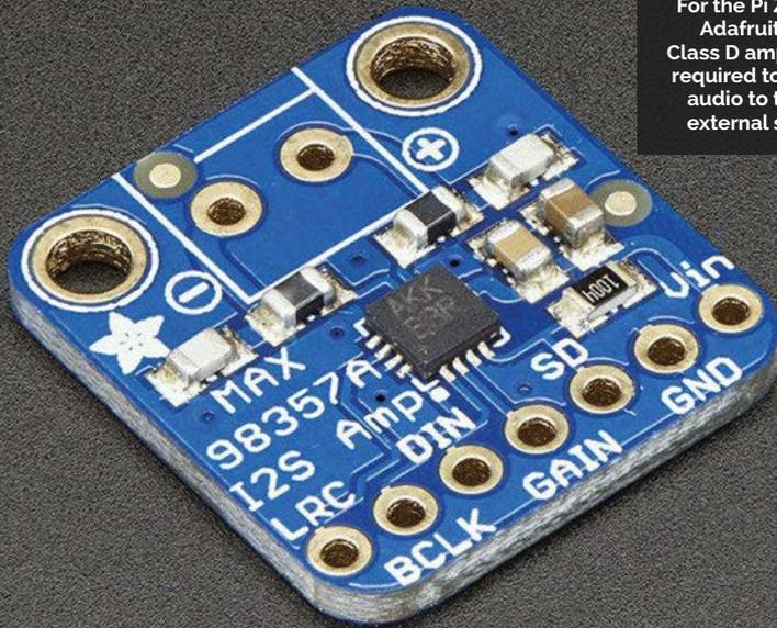
For the Pi Zero, an Adafruit I2S 3W Class D amplifier is required to supply audio to the mini external speaker
