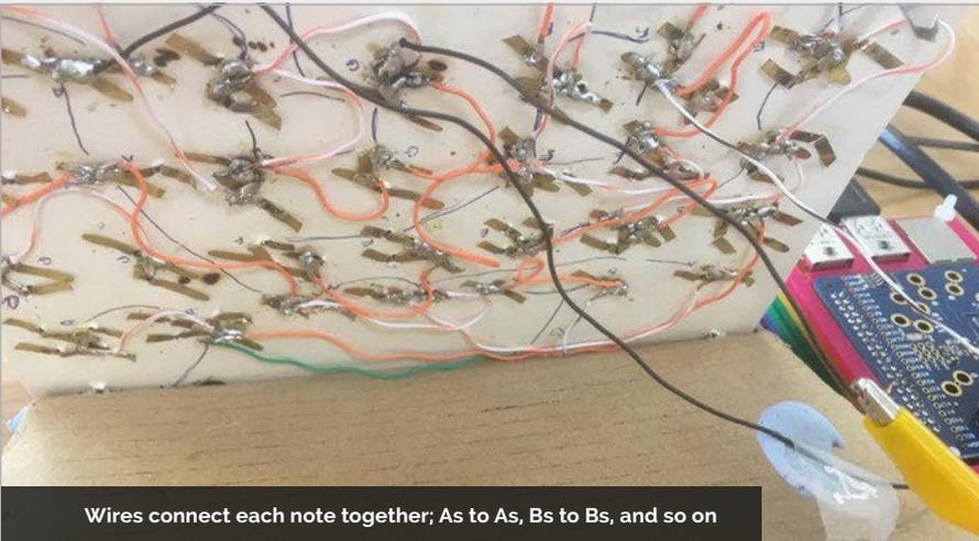
Wires connect each note together; As to As, Bs to Bs, and so on
