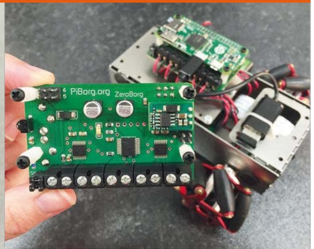
can all be powered by a standard 9V PP3 battery. Alternatively, an external power source such as a battery pack can be attached to two of the ZeroBorg's terminals, enabling you to mount it flat. The KS2 model also includes an infrared sensor (more on that later) and a second six-pin male I<sup>2</sup>C header for daisy-chaining with other add-on boards,
