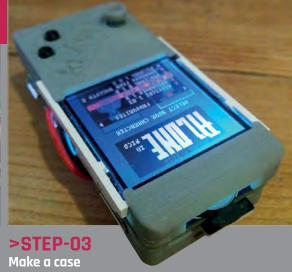
Peter designed his own slimline case using OnShape. It comprises a top, bottom, and backplate, and covers for the joystick and buttons. Find the files at magpi.cc/2quoP6f
