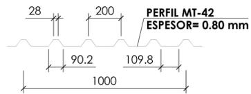
**DETALLE CHAPA CUBIERTA (h =42 mm )**
