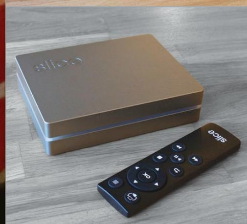
**Right** The anodised aluminium chassis houses a Raspberry Pi Compute Module, a real-time clock and can hold a slimline 3TB 2.5" hard drive
