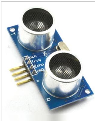
Left The HC-SR04 Ultrasonic Rangefinder. Cheap-as-chips sonar
