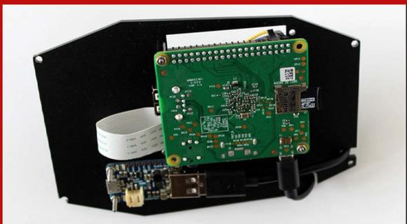
The camera case's customisable component holders are laser-cut from acrylic. "We've designed the inserts so that they perfectly fit all of the Raspberry Pi models currently available," explains Jon Fidler. "The design is very simple, using spacers, screws and nuts, making it accessible to anyone with a small screwdriver."
