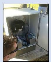
Recording equipment and back-up electricity supply for a Gulf of Corinth seismometer
