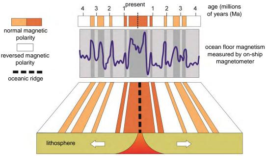
basalts erupt onto the ocean floor and take on the magnetic field of the time
