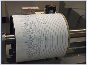
Drum record from a seismometer
