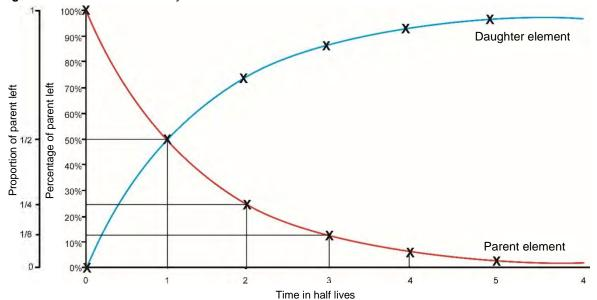
Figure 3.1. The radioactive decay curve for the breakdown of all radioactive materials
