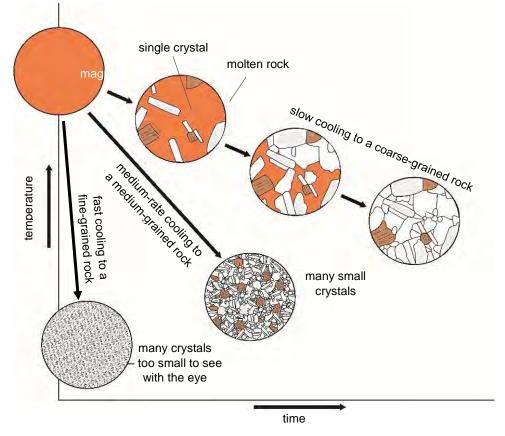
Figure 4.5. The cooling and crystallisation of igneous rocks
