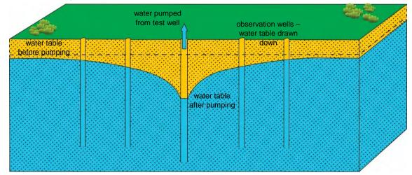
Figure 4.37. Well-testing
