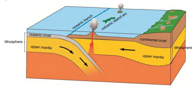
**Figure 4.25.** The Caribbean island arc, showing the curve of the deep-sea trench with the arc of volcanic islands inside, as the North Atlantic plate collides with the Caribbean plate
