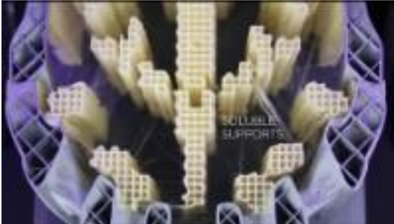
Referencia: Print complex geometries with water-soluble PVA supports - BCN3D Sigma R17 [BCN SIGMA](#)
