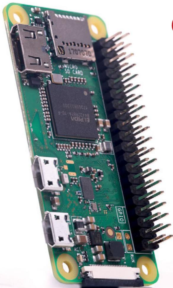
**T**he Raspberry Pi Foundation has launched a new Pi model, the Pi Zero WH. The difference between this edition and the current Pi Zero W is its pre-soldered GPIO header.
