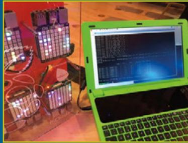
The cluster\_action script is used to control the Raspberry Pi boards
