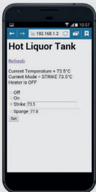
In order to control the temperature, the brewery makes use of three methods – an electronic control panel, a webpage viewable on a smartphone, and a PyQt4 GUI application – all of which can be used at the same time. Fuzzy Duck also uses software running on a Pi for its invoicing and cask tracking. That software was written using Python 2.4 in 2007, well before the Pi’s birth, however.
