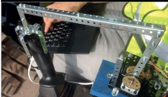
RITH developed “a solution for controlling a full-size digger with a Nod ring,” a gestural controller that fits on the finger, for *The Gadget Show*. “We created a simple servo-driven arm controlled by computer to interpret the signals coming from the ring,” Sam explains. “The digger arm essentially followed the movement of the user’s arm.”
