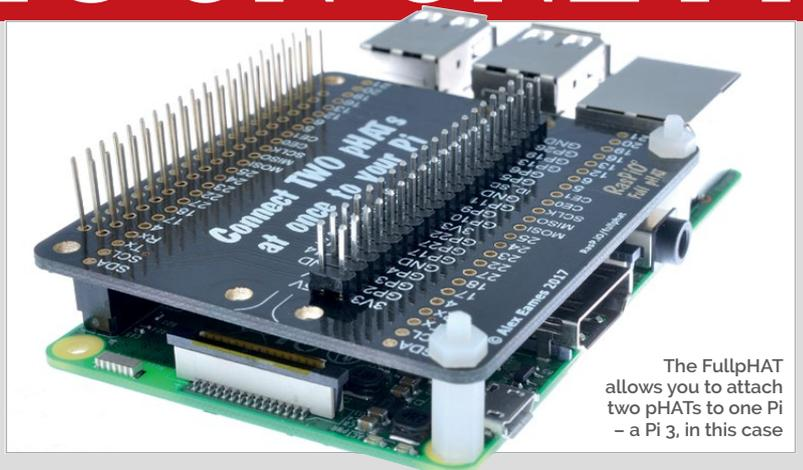
The FullpHAT allows you to attach two pHATs to one Pi – a Pi 3, in this case
