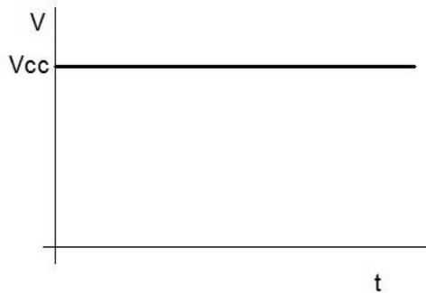
DC - 100%:  $V_{med} = V_{cc}$
