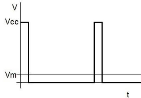
DC - 10%:  $V_{med} = V_{cc}/10$
