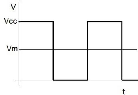
DC - 50%:  $V_{med} = V_{cc}/2$
